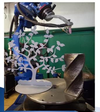
The tree was plasma cut from 1.5 mm thick mild steel sheet. The robot job was generat from a DXF file using Sprutcam.
